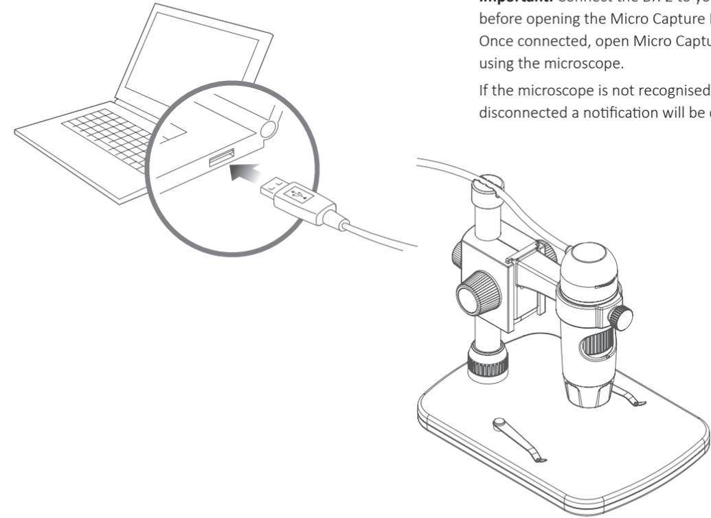
**Important:** Connect the DX-2 to your computer before opening the Micro Capture Plus software. Once connected, open Micro Capture Plus to start using the microscope.
