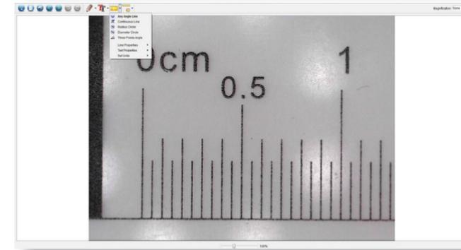
**Step 3** Once the image is open, click on the calibration icon. Using the mouse, click on the beginning and ending points; you must know the distance between the points (using the ruler). A dialogue box will pop up, enter the exact value of the measurement into 'Actual dimension'. The software will automatically calibrate the magnification rate. Click 'OK' and the adjusted magnification rate will show in the upper right corner.
