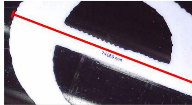
**Diameter Circle Measurement** Click, hold and extend out to the chosen diameter. The diameter, circumference and area of the circle will be calculated.
