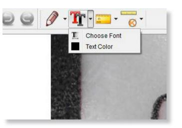
You can annotate captured images using the draw or add text features; this is useful when using for later analysis.
