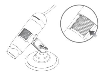
To focus the microscope rotate the focus wheel on the front of the microscope; clockwise to zoom-in or anti-clockwise to zoom out. Using the software, you will be able to see on screen whether the DX-1 is focused. Capture a still photo or video footage at any point when using the microscope, use the icons or dropdown menu within the Micro Capture Plus software.
