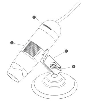
**Focus Wheel** Adjusts the focus of the microscope on the object
