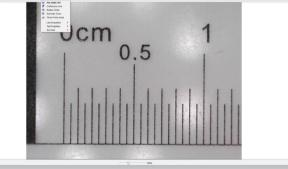
**Step 3** Once the image is open, click on the calibration icon. Using the mouse, click on the beginning and ending points; you must know the distance between the points (using the ruler). A dialogue box will pop up, enter the exact value of the measurement into 'Actual dimension'. The software will automatically calibrate the magnification rate. Click 'OK' and the adjusted magnification rate will show in the upper right corner.
